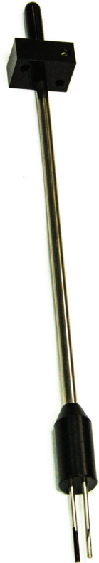
Each probe of the REMS electrode contains a pair of electrodes for injecting current and measuring voltage.
